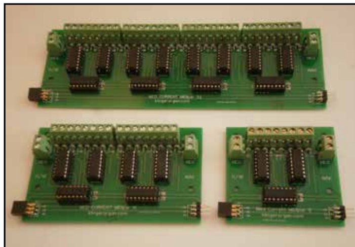
Medium Current boards. Maximum 1.5 A per driver output.
