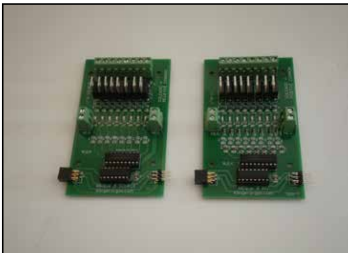
High Current boards. Maximum 5 A per driver output
